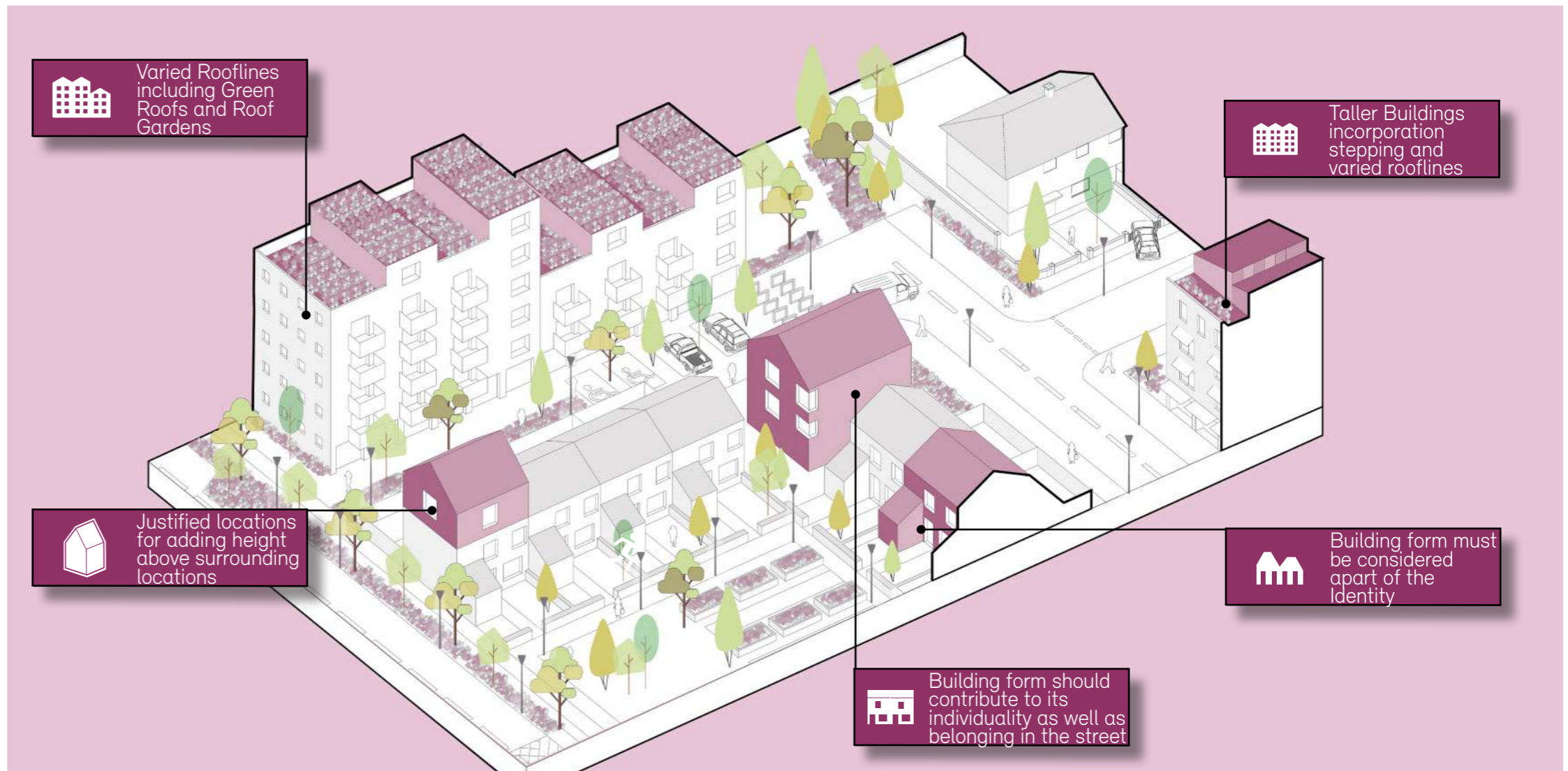
Illustrative diagram showing scale and form principles
